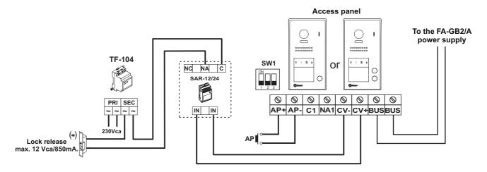
(\*) Important: Fit the varistor supplied with the kit directly to the terminals of the lock release.
