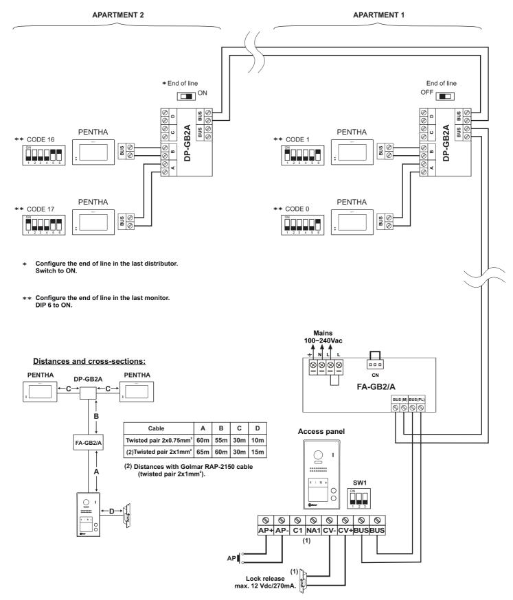
(1) Important: For AC lock release, 2nd AC lock release or automatic gate, see wiring diagrams p. 22.
