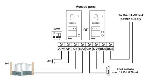
(\*) - To switch voltages higher than 12Vdc/1A between terminals 'C1' and 'NA1' on the door panel, consult our technical support service. - 'C1' and 'NA1' potential-free contact.
