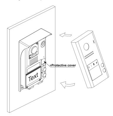
To finish the mounting of the door panel, replace the metal front.
