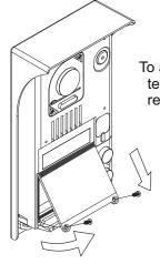
To access the connection terminals, remove the card reader.
