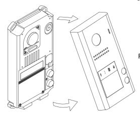
Remove the metal front as shown in the drawing.
