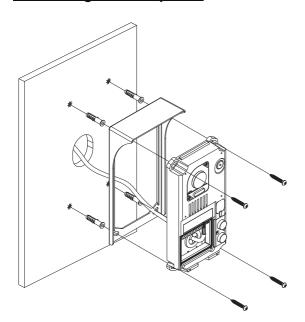
Present the shield and the electronic module to the wall, placing the top of the module at a height of 1.65m from the ground, and pass the wiring through the cable entry.
