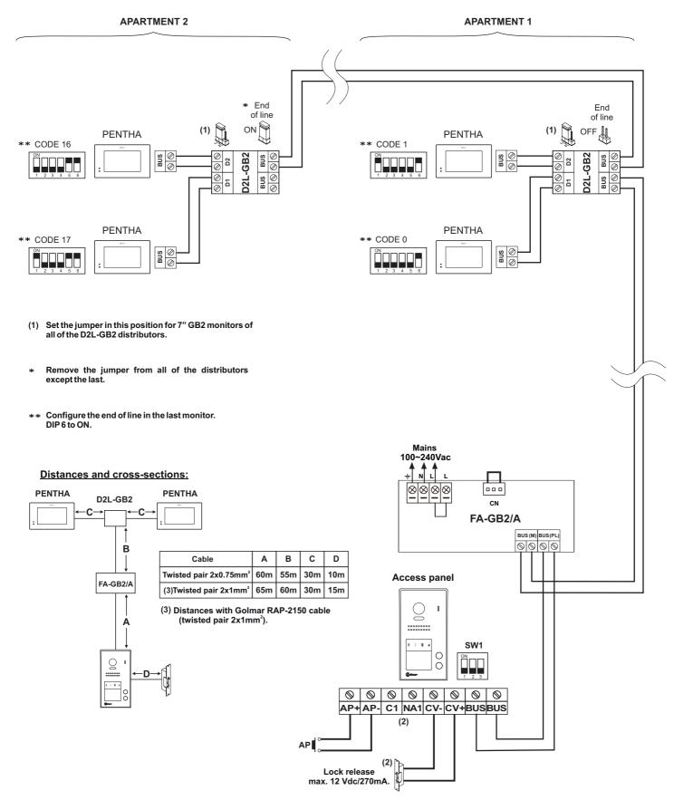
(2) Important: For AC lock release, 2nd AC lock release or automatic gate, see wiring diagrams p. 22.
