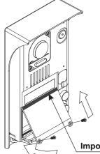
After completing the wiring and configuration work, position the nameplate label in the electronic module. Fix using the screws supplied.
