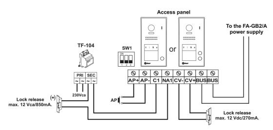
(\*) Important: Fit the varistor supplied with the kit directly to the terminals of the lock release.
